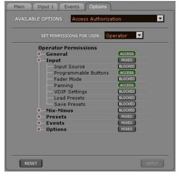
To log in to a given mode, press the button on the lower left corner of the VGA screen that displays the current ACCESS AUTHORIZATION level.
