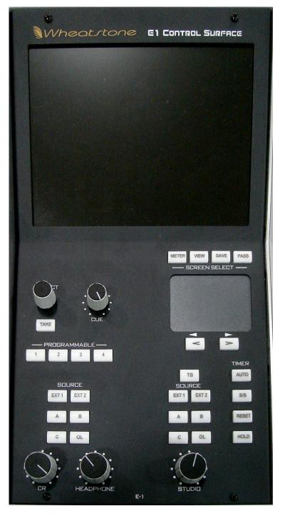
• When no A/B button is lit, pressing the SELECT knob will open a screen showing a full list of input sources and locations for quick source selection on a fader, or for making other connections within the system. This operation may be denied to a user in the Access Authorization settings.
