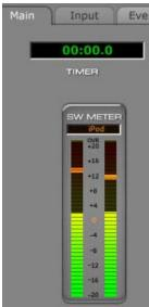
The switched meter display shows the signal source name at the top. Click on this name to bring up the source selection window and change the signal as desired.
