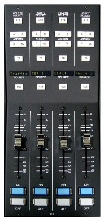
Press the fader's A/B switch and hold it until the button lights (as opposed to tapping it for source switching). This switches the VGA screen to the *Input* tab for this fader, where you can change the programmed sources for A and B, select the fader mode, adjust panning, and set up VDip. All of these functions are covered in the following paragraphs, with the exception of VDip, which is discussed in the next chapter on the master panel.
