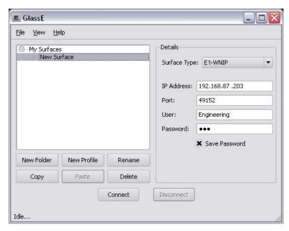
Select the Surface Type, enter the surface's IP address, and enter the Port you previously set up at the E-1. Then enter the user name and password that corresponds
