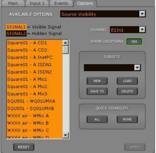
With this form the user can set the channel's source visibilities. Scroll up and down the source list and highlight the desired source signal(s) and click the *APPLY* button to save the visibility options. If you have made changes and then decided you don't want to put the changes into effect, click RESET. This will cancel any changes you made since entering the screen or since clicking APPLY, whichever happened most recently.
